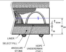
$$H_{gw} \times (62.4 \text{ lb/ft}^3) = [(Y_{stone} \times t) + [(Y_{fill} \times t)] / SF$$
