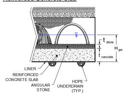
Alternatively, an engineer can design a reinforced concrete slab. The slab should be designed to handle the uplift forces from groundwater while transferring live & dead loads to the underlying material.
