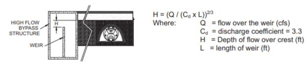
In a typical downstream overflow design, the designer may incorporate one or more low flow orifices into the high flow weir wall. The weir crest is established as described above but hydraulic losses from the inlet to chamber to the outlet structure may need to be considered. Losses may be factored in by lowering the weir crest or increasing the liner freeboard.
